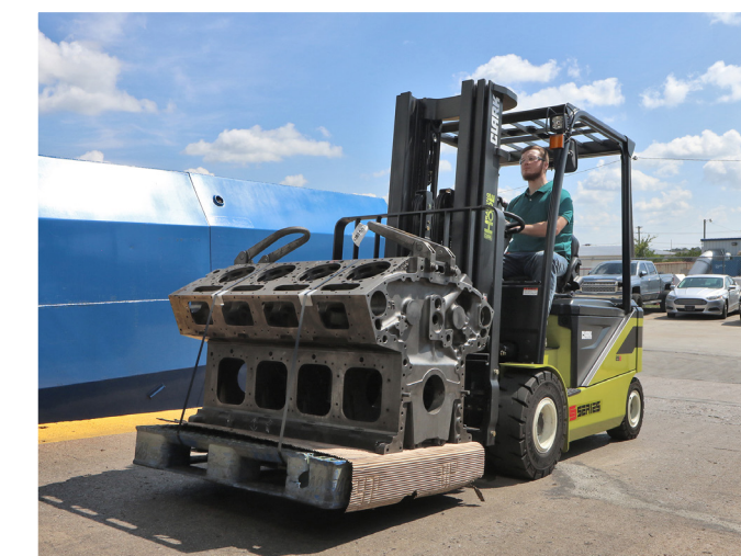
0° ZERO TURN STEER AXLE Turning Radius Minimum of 76.5" (1943mm)
