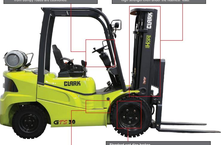
Driver accesses the ergonomically designed compartment via a large, low, perforated non-slip metal step.
